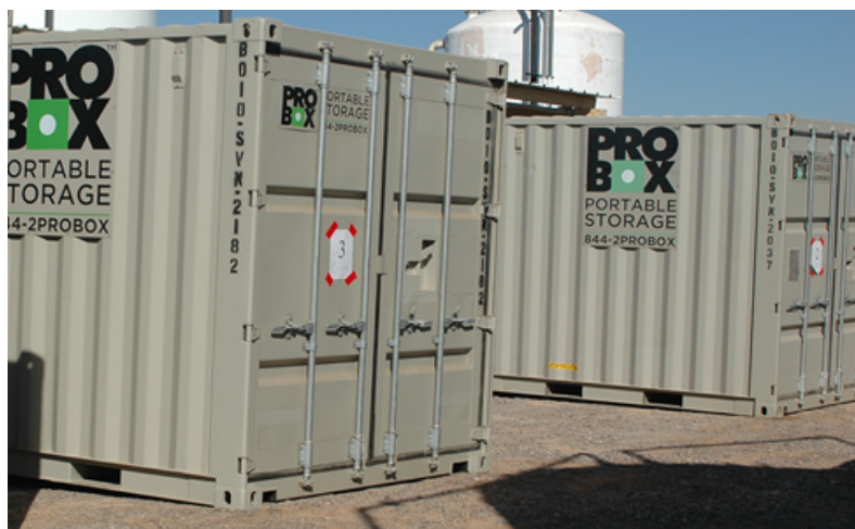
Figure 2. Commercial storage containers used in these studies, each a 10 ft cube with steel walls & wooden floors.
