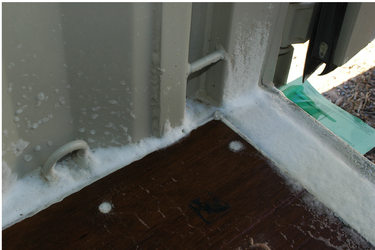
Figure 7. Foaming at full or diluted concentrations had the advantage of coating all surfaces and seeping into potential pest harborages like under the door jam, rubber gasket. Note the coat of foam still visible in Experiment 3 2.5 h after foaming in the door threshold (right).
